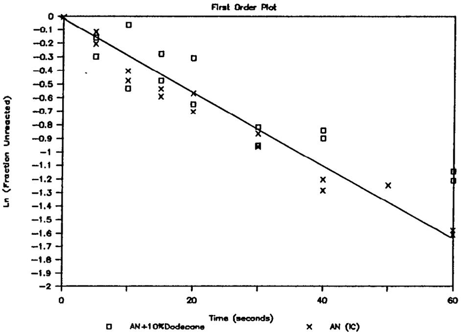
Fig. 3. First-order plots of the thermolysis of a slurry of ammonium nitrate with 10 wt.% *n*-dodecane at 250 and 340°C compared with ammonium nitrate decomposition at those temperatures.
