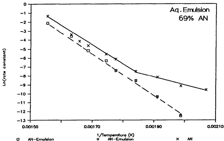
Fig. 5. Arrhenius plot of the thermolysis of the aqueous emulsion (dashed line) and of neat ammonium nitrate (solid line).
