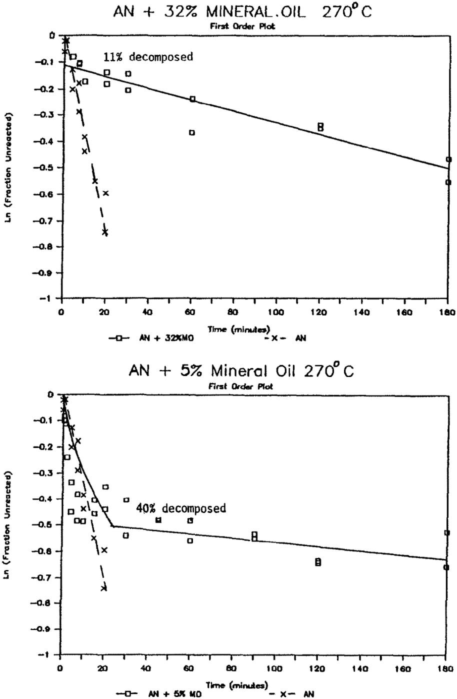
Fig. 10. First-order plots of the thermolysis at 270 °C of a slurry of ammonium nitrate with 5 wt.% and with 32 wt.% mineral oil. (Ammonium nitrate thermal decomposition indicated by --X--).
