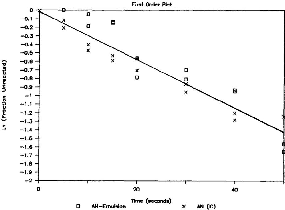
Fig. 2. First-order plots for thermolysis of the aqueous emulsion at 250 and 340°C compared with ammonium nitrate decomposition at those temperatures.
