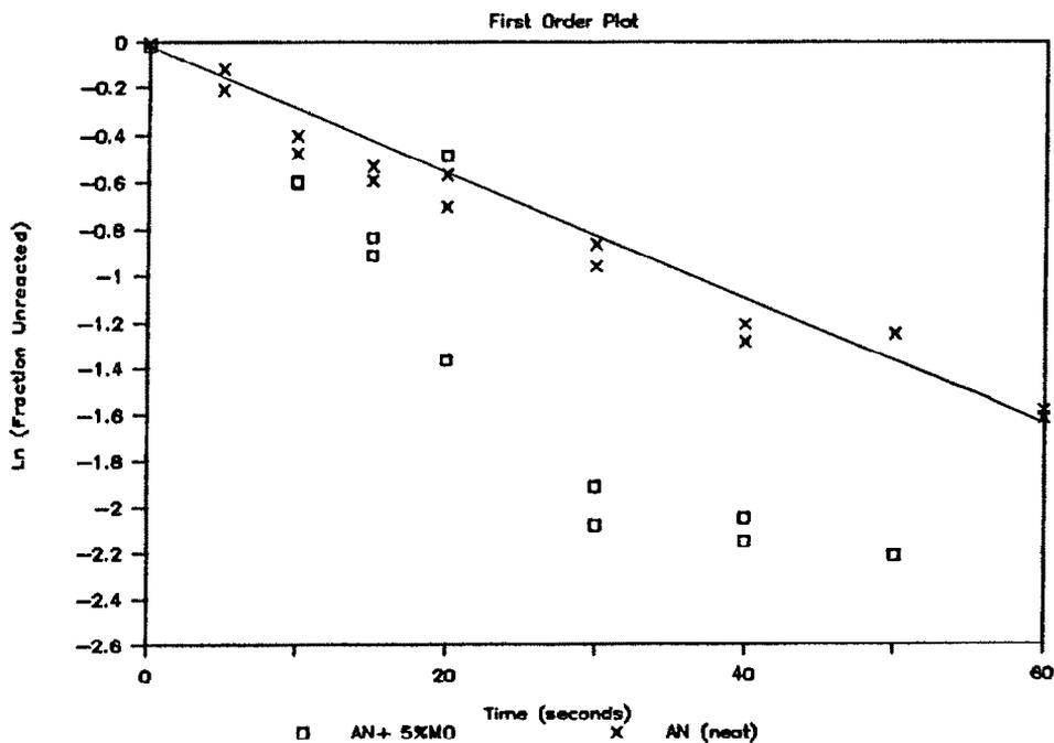
Fig. 4. First-order plots of the thermolysis of a slurry of ammonium nitrate with 5 wt.% mineral oil at 250 and 340°C compared with ammonium nitrate decomposition at those temperatures.
