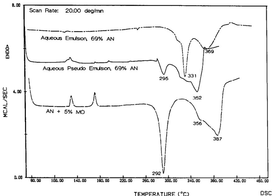
Fig. 9. Thermograms of ammonium nitrate with 5 wt.% mineral oil, an aqueous emulsion, and a pseudo-emulsion, scanned  $20^{\circ}\text{C min}^{-1}$ .
