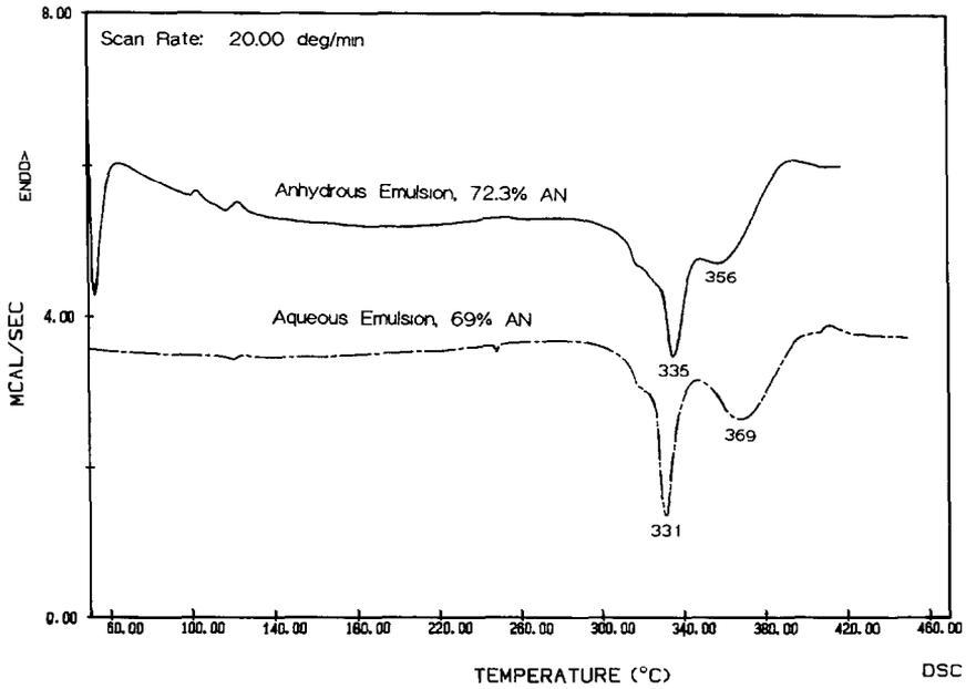
Fig. 8. Thermograms of the aqueous and anhydrous emulsions, scanned  $20^{\circ}\text{C min}^{-1}$ .
