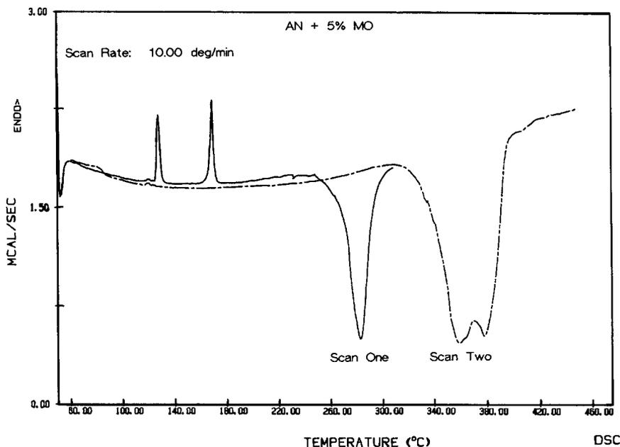
Fig. 11. Thermogram of ammonium nitrate with 5 wt.% mineral oil scanned to 315°C (Scan One, solid line), cooled, and rescanned (Scan Two, dashed line); scans at 10°C min<sup>-1</sup>.
