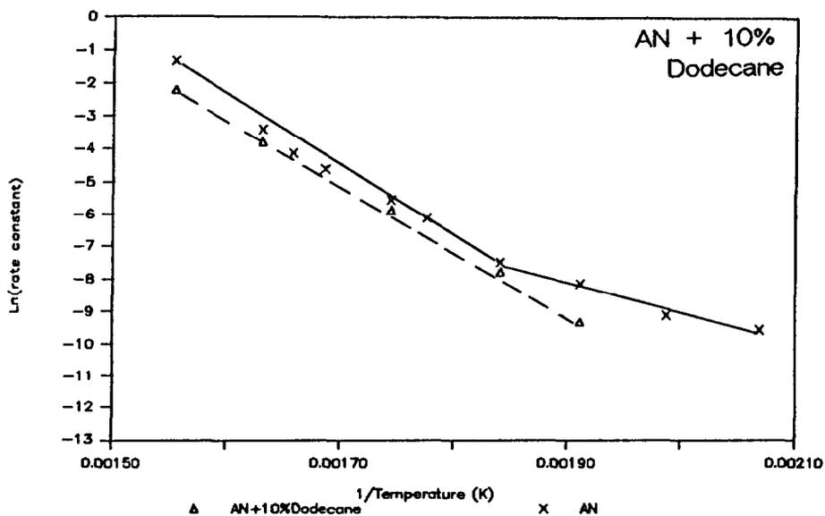
Fig. 6. Arrhenius plot of the thermolysis of a slurry of ammonium nitrate with 10 wt.% *n*-dodecane (dashed line) and of neat ammonium nitrate (solid line).
