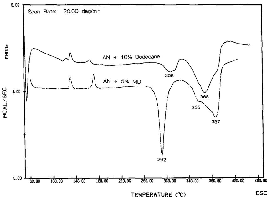
Fig. 12. Thermograms of ammonium nitrate with 5 wt.% mineral oil (dashed line), and ammonium nitrate with 10 wt.% *n*-dodecane (solid line), scanned  $20^{\circ}\text{C min}^{-1}$ .
