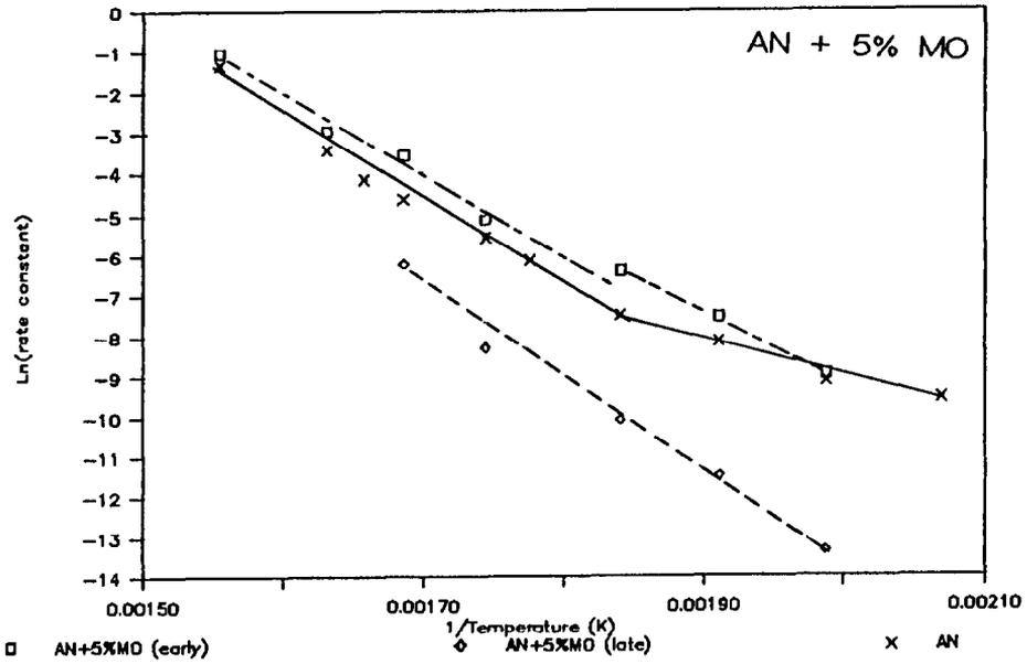
Fig. 7. Arrhenius plot of the thermolysis of a slurry of ammonium nitrate with 5 wt.% mineral oil (dashed lines) and of neat ammonium nitrate (solid line).
