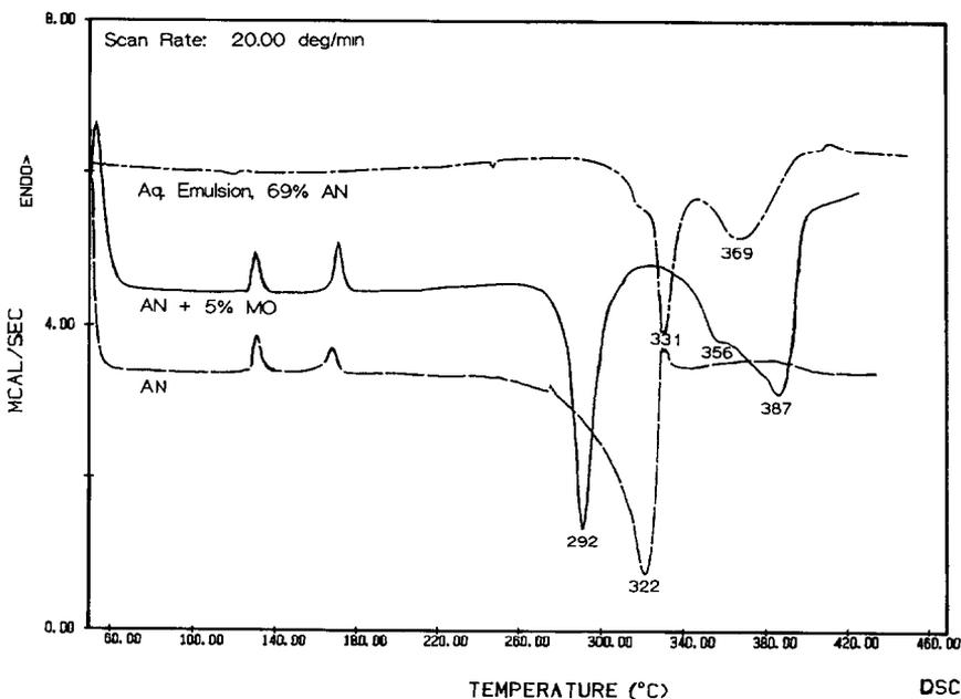
Fig. 1. Thermograms of ammonium nitrate, ammonium nitrate with 5 wt.% mineral oil, and aqueous emulsion, scanned  $20^{\circ}\text{C min}^{-1}$ .
